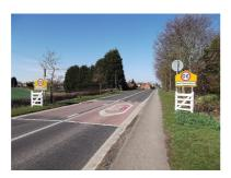
b. Solar-powered 'Vehicle Activated Signs.' Approx £2500-£2750 for Sign and £1155 for the solar panel (all installed). Note – any potential new speed limit in future would require a new sign (at cost). OCC Highways would typically fund and install VAS pole.
